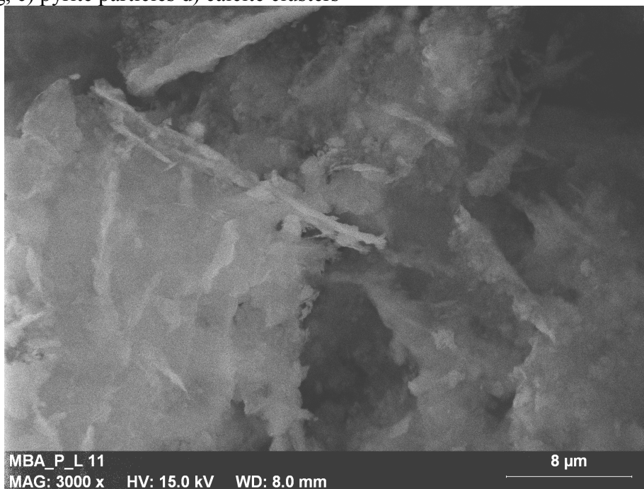
Fig.10. SEM micrograph of purified MBA (MBAp): curved, exfoliated clayey layers
