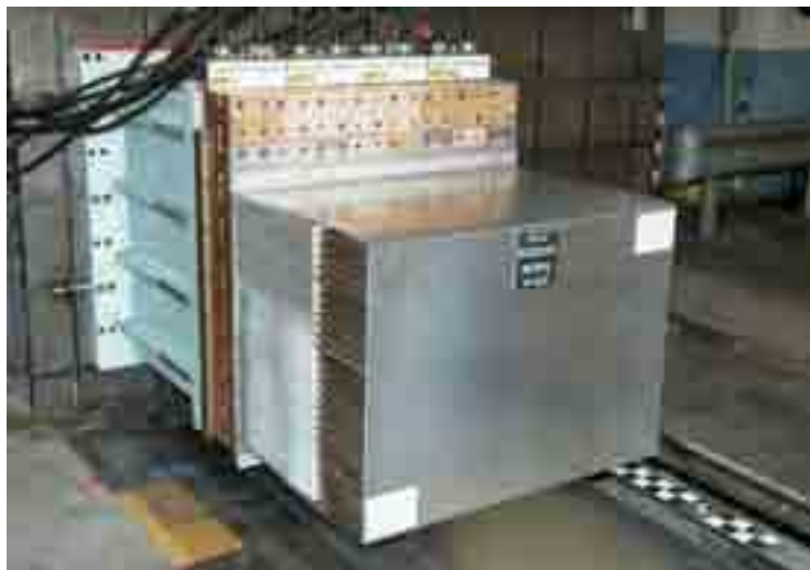
Figure 1: PDB barrier V7 mounted on a HRLCW
